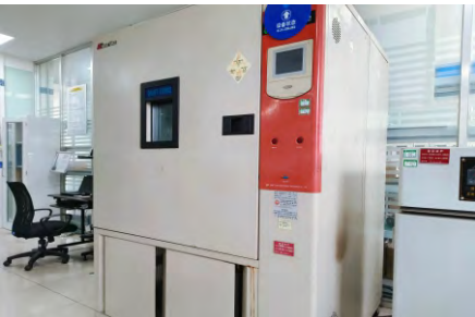
Constant Temperature and Humidity Test Chamber
