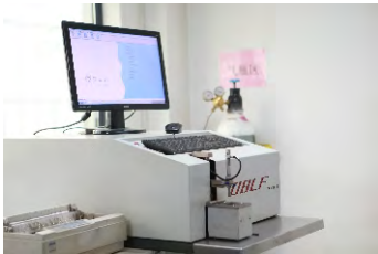
Chemical Analysis before Pouring
