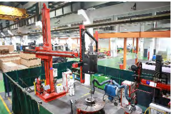
Hot-wire TIG Automatic Cladding System
